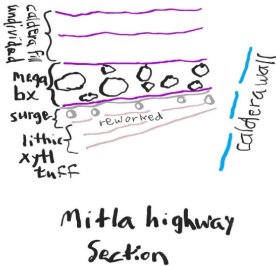
Figure 7.8. Schematic stratigraphic section of caldera-related volcanic rocks, Rama de Oro project.
